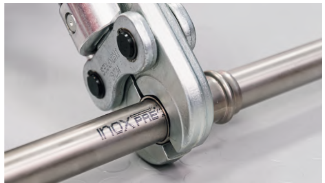
Figure 25 - Making the press connection
