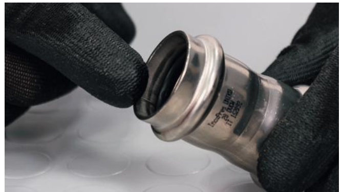
Figure 23 - Checking the sealing ring
