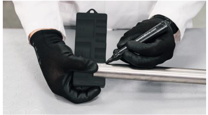
Figure 22 - Marking the insertion depth
